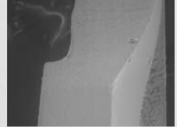
C- Edge profile at Optic-haptic junction. Radius of curvature <10\mu\text{m} .
