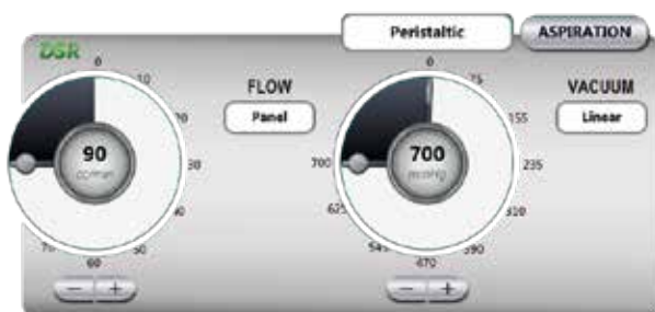
PERISTALTIC PUMP Flow rate: up to 90 cc/min Vacuum: up to 700 mmHg
